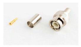
Conductor pin size, External width 2.1mm, Internal conductor hole 0.9mm Will fit variations of RG59 Coax Cable with conductor core 0.5mm – 0.88mm
